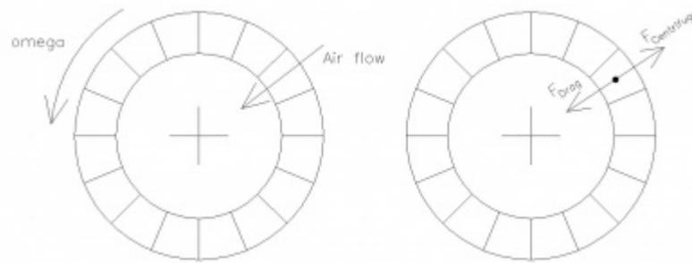
A dust cloud is created from the fed powder. Due to under-pressure inside air flows through the rotating classifier. Smaller particles are removed from the cloud by the air flow. The large particles remain outside the classifier. Both fractions are collected in bins.
