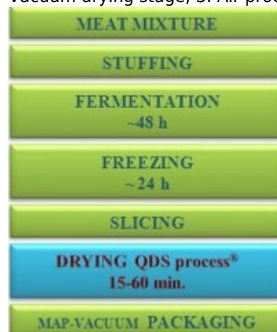
Fig.2. Diagram of the processing steps for the production of a stuffed fermented product dried by means of the "QDS process®"; © IRTA
