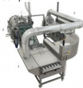
Fig.1. "QDS process®" pilot equipment: 1. Tempering/convective drying stage; 2. Vacuum drying stage; 3. Air processing circuit with HEPA filter; © Metalquimia S.A.
